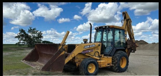
JOHN DEERE 710D BACKHOE
